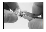
Verify that the wires are still correctly aligned to the pattern. Slide the \$45-1755P metal shell over the plug body as shown above. Press-In on the bottom of the plug as you attach the shell. This will allow the plug to snap into the metal shell. The drain wire should remain straight back against the cable jacket and come out of the back of the metal shell and extend pass the external ground arm.
