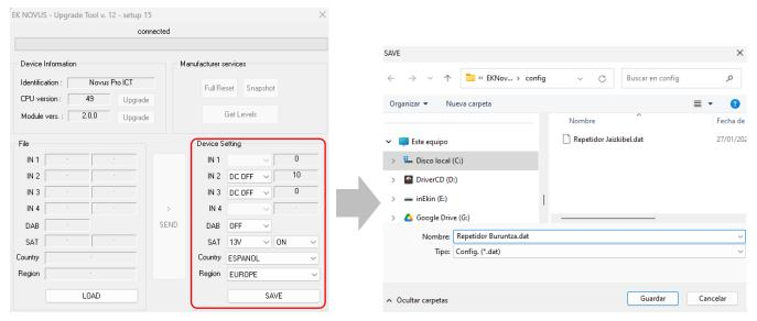
To copy one of the saved settings to another programmable amplifier, select the desired file using the LOAD button:
