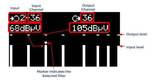
By pressing the center button, you can directly access the EDIT menu of the selected filter using the marker.
