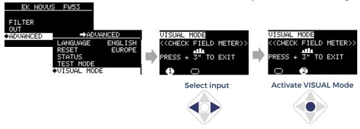
By activating VISUAL mode with a central click, the selected channel begins to flash on the field meter, making it easier to visually identify. Using the joystick's directional keys, you can change the frequency, adjust the output level, or remove the filter. With another central press, the next higher frequency channel is selected.
